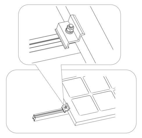
Turn the module and locate the hole in the rear frame. Use the tooth of the railing hook to fix it to the frame and secure it with an M8x25 screw and nut.
