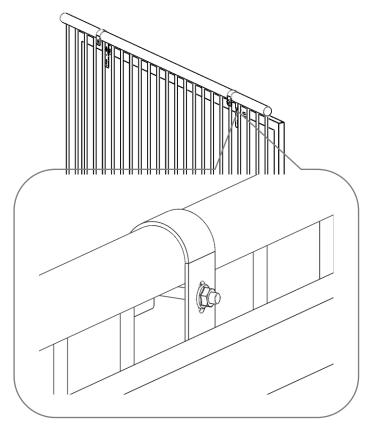
Insert the T-bolts into the groove in the rails and fix the lower part of the module to the balcony railing using the fixing plate and nuts.
