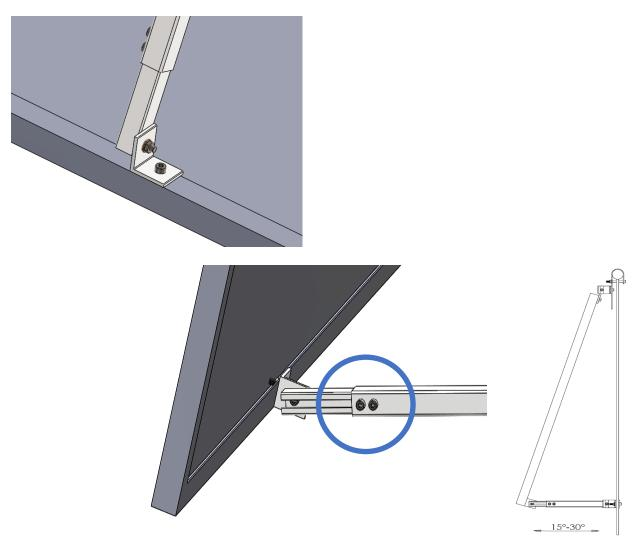
Then fix the poles to the balcony railing by using the screws M8 x 45 and nuts. Finally, secure the upper brackets by using the metal ribbons.
