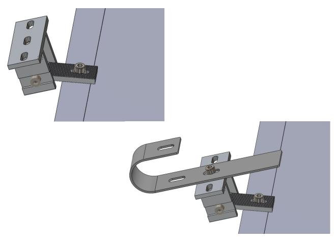
Hang-up the PV module on the balcony railing and secure the railing hooks with the M8  $\times$  75 screws and nuts.
